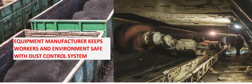
**Problem:** A leading manufacturer of bulk handling equipment in Brazil needed a system to control iron ore dust. When customers use the rail cars, they are inverted for unloading so the iron falls from the cars into chutes. The manufacturer's customers could be jeopardizing the health of its employees and facing significant environmental fines without effective dust control.
